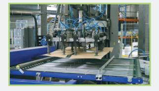
The Palcut Dispenser is a fully automated dispenser which cuts Caregrip paper to the desired length from a roll.
